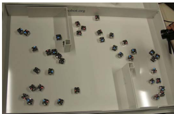
Fig. 5. An experiment run with about 40 robots. Wall sections in the field prevent that robots uniformly follow the walls. Gender and life status are indicated with colored LEDs.
